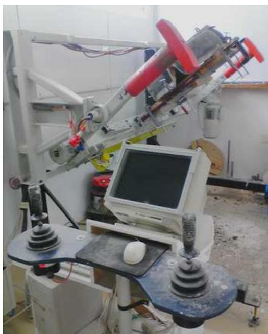
Experimental two-axis casting machine with computer to program specific flow
